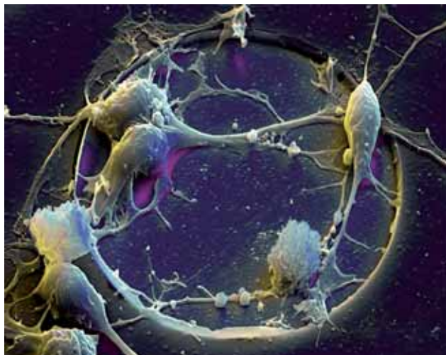
Nerve cells cultured on a micro-electrode chip for testing analgetics. (Foto C. and M. Kage)
