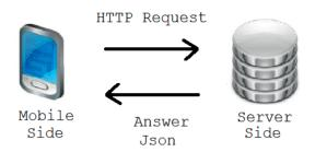
Fig.1. Interaction between the server side and the Mobile side.
