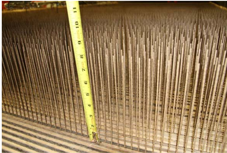
Figure 1. Picture of laser-cut cardboard laboratory fuel bed. Note that the scale is graduated in inches.
