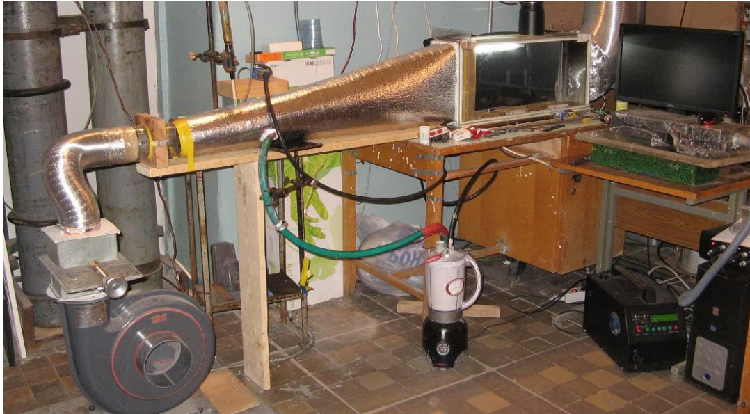
Figure 2. Experimental setup for measuring the flame spread velocity across pine needles bed
