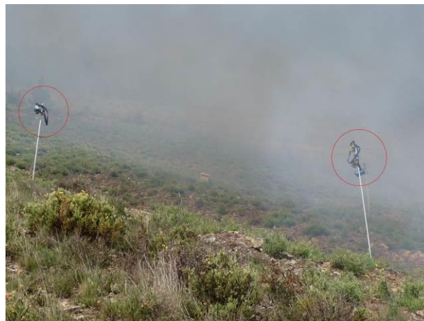
Figure 4. PM 2.5 monitoring sensors indicated by the circles.
