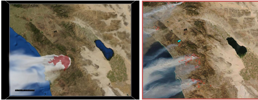
Figure 4. Smoke dispersion within domain D03 (2km resolution) simulated by WRFSC (left panel) and MODIS satellite image (right panel). The red color fill in left panel represents the fire area projected from the nested fire domain D04 (500m resolution). Red contours in right panel represent remotely detected hot spots.
