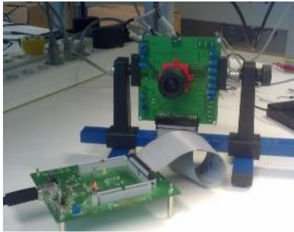
Figure 3—Experimental setup: vision sensor and data logger.
