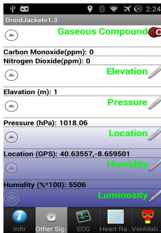
Figure 5 –Improved DroidJacket Version.
