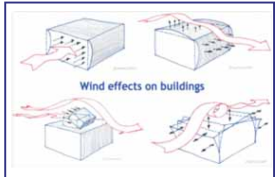
Fig. 30: Shown in this figure clockwise from top left are the following effects of wind as it interacts with a building: (a) Positive wind-velocity pressure; (b) Negative (suction) wind-velocity pressure; (c) Buffeting, and (d) Leveling-off also known as 'clean-off' effect.
