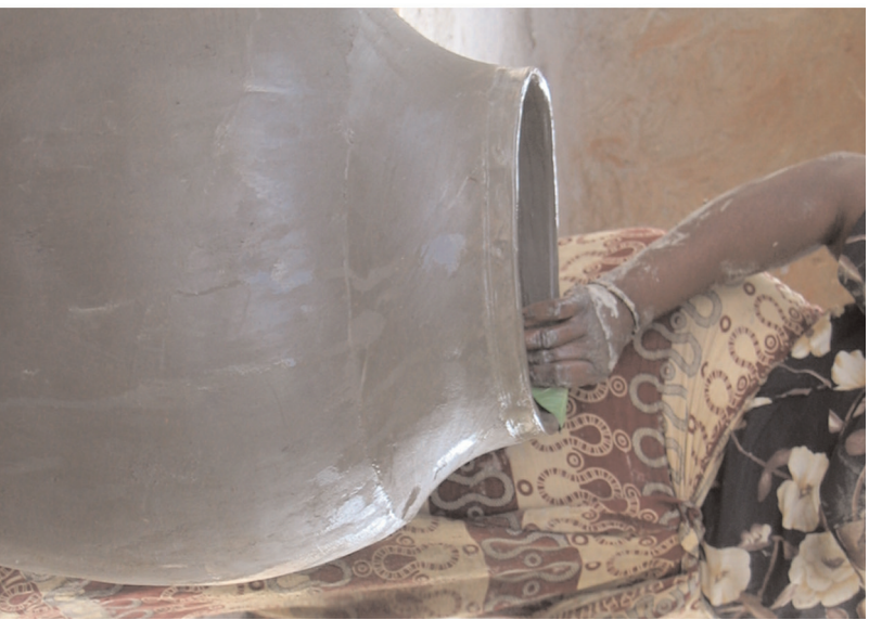
FOTO 6 – Smoothing the lip of a vessel
