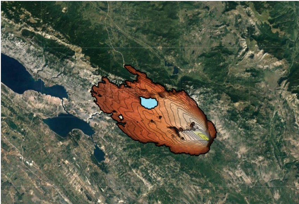
Figure 3 - AdriaFirePropagator simulation - blue area represents fire barrier (non burnable area).
