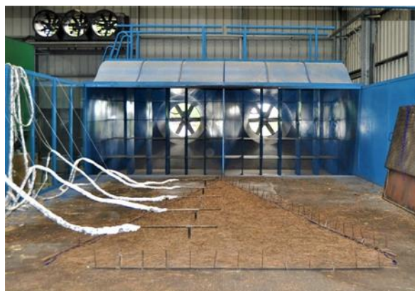
Figure 2 - wind tunnel of LEIF
