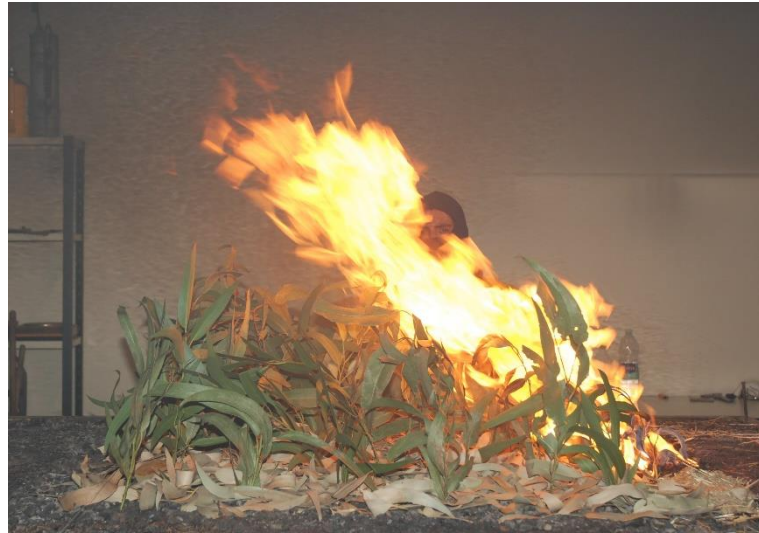
Figure 1 - Wind-driven fire spread test in a fuel bed of Eucalyptus globulus leaves litter over layered by quasi-live E. globulus twigs.
