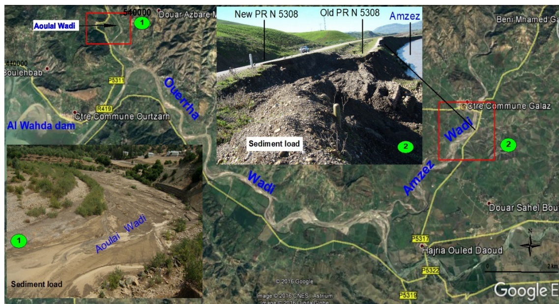
Figure 13 Solid sediment load produced by the hydrodynamic actions and leads directly into the Al Wahda dam in Rif mountains. Source: Background from Google Earth 2016, and field trip in May 2017.
