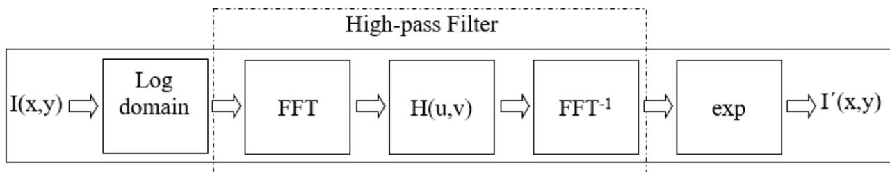
Figure 1 - Homomorphic filtering process in frequency domain
