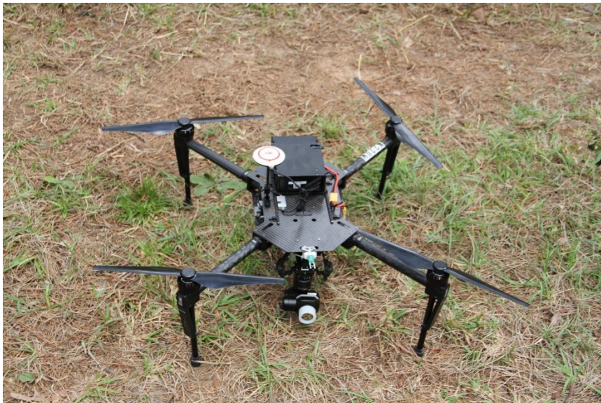
Figure 3 - DJI matrice UAS with FLIR Zenmuse XT infrared camera.
