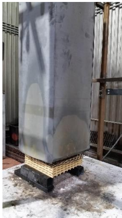
Figure 1 - Crib design #3 under 3.66 m tall chimney.
