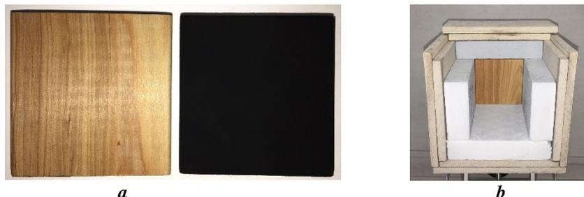
Figure 2 - a) Original (left) and blackened (right) sample; b) sample holder to block convection cooling
