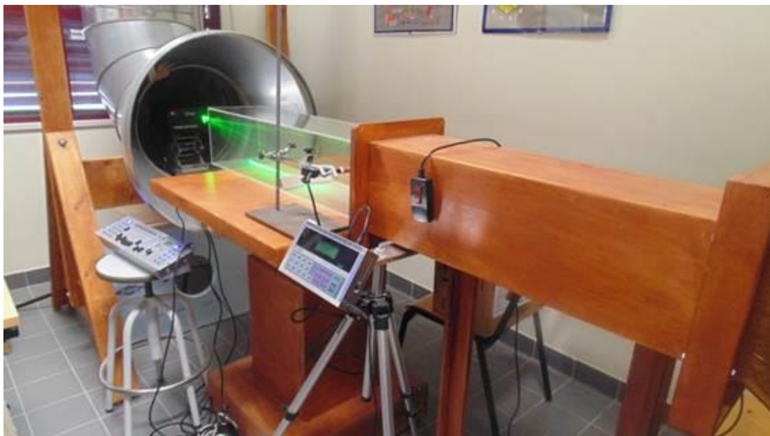
Figure 1 - Scheme of the low air velocity aerodynamic tunnel, test section and laser used in the experimental tests.
