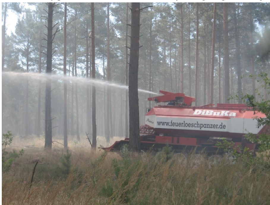
Figure 3 - Fire tank in action
