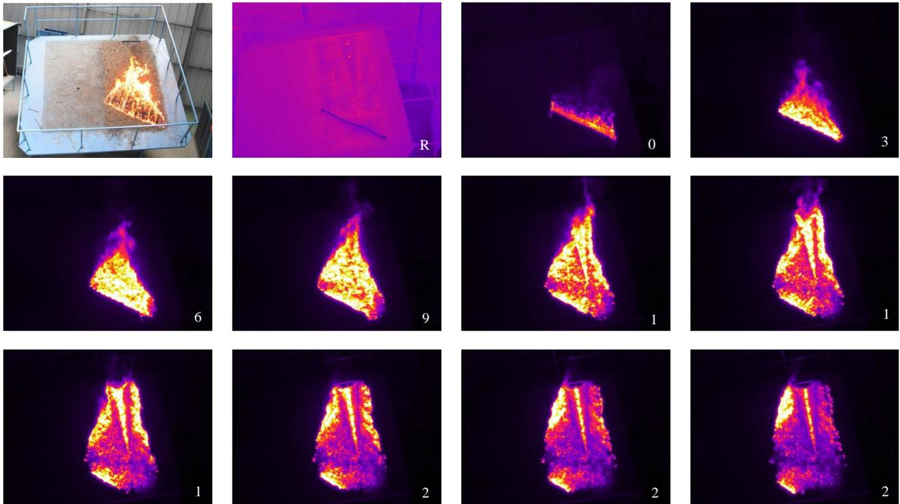
Figure 5 - Test AVE08 ( $\alpha=30^\circ$ ;  $\gamma=20^\circ$ ;  $\delta=45^\circ$ ): visible picture of the table, reference frame and frames every 30 seconds, from instant 0s to 270s.
