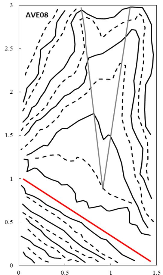
Figure 6 - Fire spread propagation contours of the AVE 08 test ( $\alpha=30^\circ$ ;  $\gamma=20^\circ$ ;  $\delta=45^\circ$ ) as a function of time (interval between 30-second contours).
