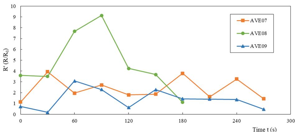
Figure 8 - Non-dimensional rate of spread along the axis of the canyon of the tests AVE07 ( $\alpha=30^\circ$ ,  $\gamma=-20^\circ$ ,  $\delta=45^\circ$ ), AVE08 ( $\alpha=30^\circ$ ,  $\gamma=20^\circ$ ,  $\delta=45^\circ$ ) and AVE09 ( $\alpha=30^\circ$ ,  $\gamma=0^\circ$ ,  $\delta=45^\circ$ ) as a function of time.
