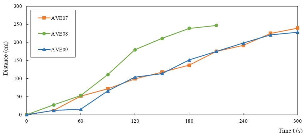
Figure 7 - Distance travelled by the fire front of the tests AVE07 ( $\alpha=30^\circ$ ,  $\gamma=-20^\circ$ ,  $\delta=45^\circ$ ), AVE08 ( $\alpha=30^\circ$ ,  $\gamma=20^\circ$ ,  $\delta=45^\circ$ ) and AVE09 ( $\alpha=30^\circ$ ,  $\gamma=0^\circ$ ,  $\delta=45^\circ$ ) as a function of time.
