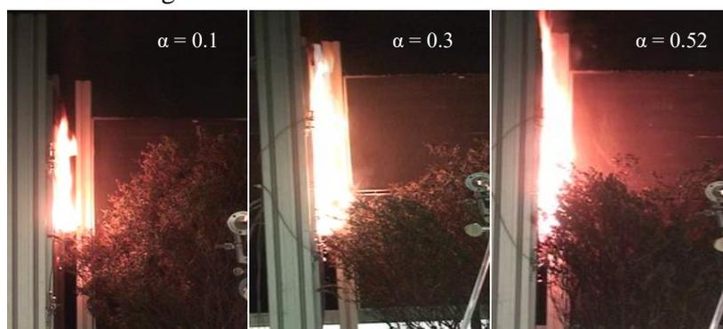
Figure 6 - Position of the ignition point in the shrub a) top of the crown, b) in the crown, c) at the bottom of the crown
