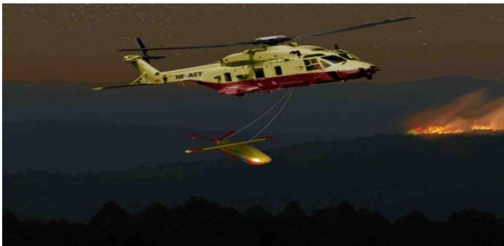
*Figure 4 - Launching of AGSs from the LA (heavy cargo helicopter) at night*
