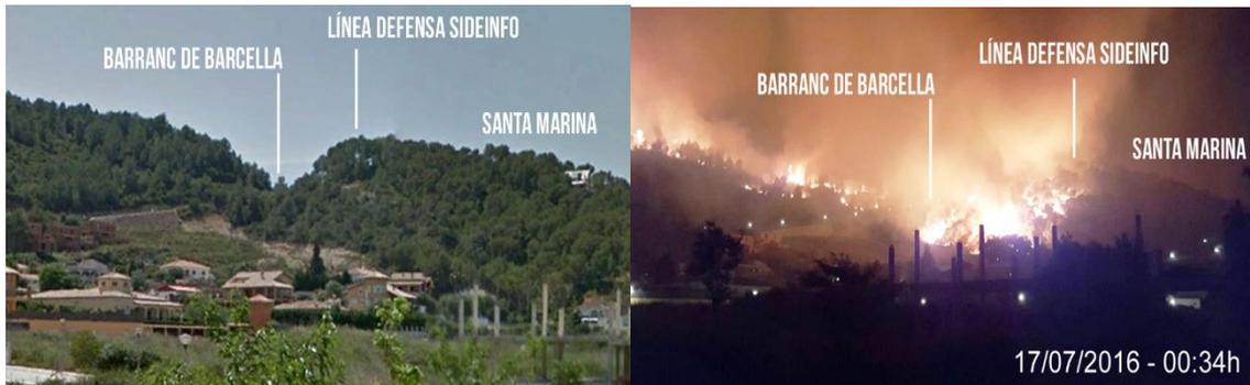
*Figure 2 - Impact in area 1 (south-east). Images taken from the position of the Advanced Command Post. In the central part of the right image certain alignment is observed. When fire reaches the top of the slope, it meets the first wetted area by the WUI-PROTECT® and stops its progression. Source: Own elaboration based on Medi XXI GSA images.*
