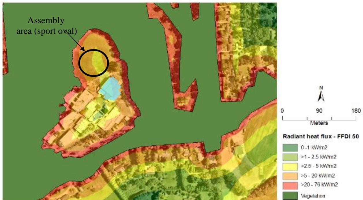
Figure 4 - Radiant heat flux exposure for FFDI 50.
