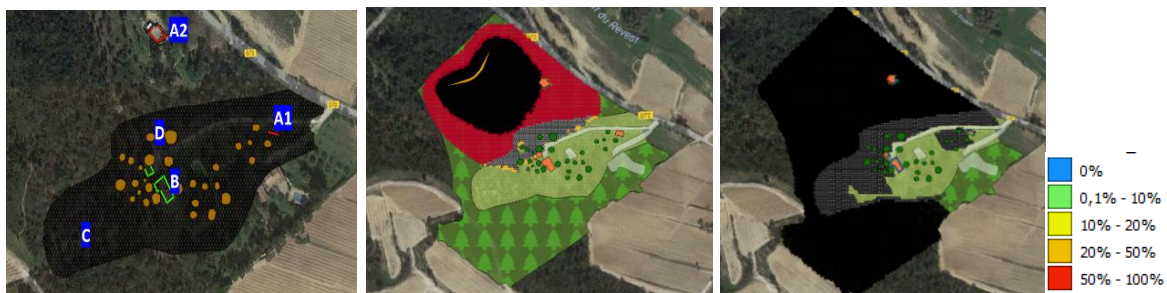
Figure 8 - Vidauban fire: comparison between the observed (left) and predicted (middle and right) damages (for color code see caption of Figure ).
