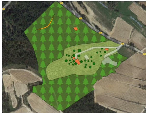
Figure 7 - Vidauban fire: visualization of the initial fire front position and the different polygons used to model the areas covered with natural and ornamental vegetation (in green), those composed of non-combustible (in grey: swimming-pool, concrete areas, etc.) and combustible (in orange) materials.
