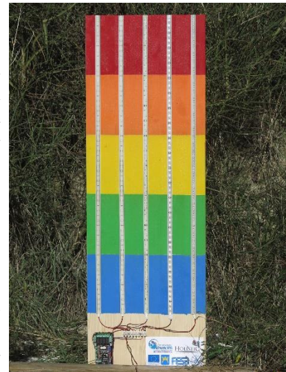
Figure 6 - Setup for LED visibility testing
