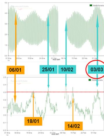
Figure 3: Sea level (upper panel) and non tidal residuals (surges, lower panel) measured in the tide gauge of Bilbao from January 1<sup>st</sup> to March 5<sup>th</sup>.
