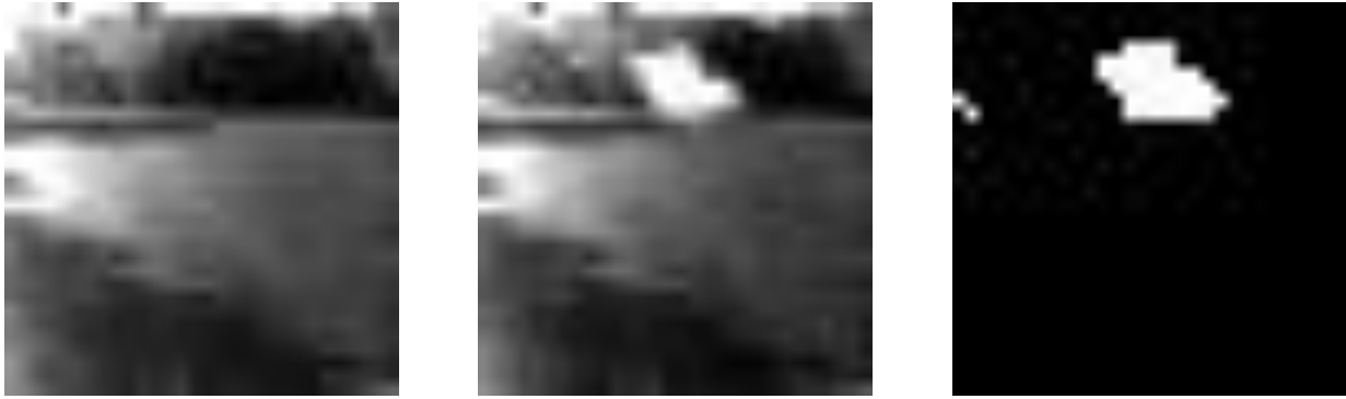
Figure 7. Background model (left), captured image (center) and foreground segmentation (right) just at the detection instant of smoke from pyrotechnic material with Silicam.
