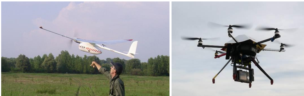
Figure 6. Launch of fix wing UAS (Fenix) for fire reconnaissance before starting intervention. Rotary wings UAS (Bee) hovering at forest fire. Source: 6DOF (Croatia) and R-Fire Ltd. (Hungary)
