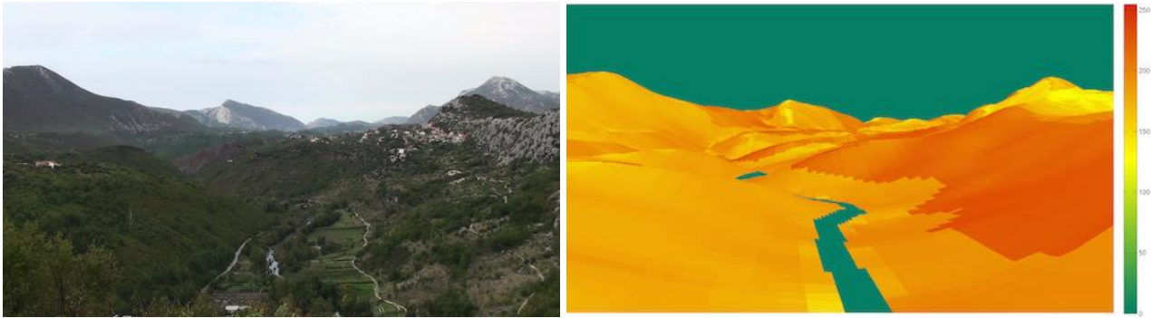
Figure 3. Original image of detection area and synthetic AR image of the same view with superimposed site-specific wildfire risk index
