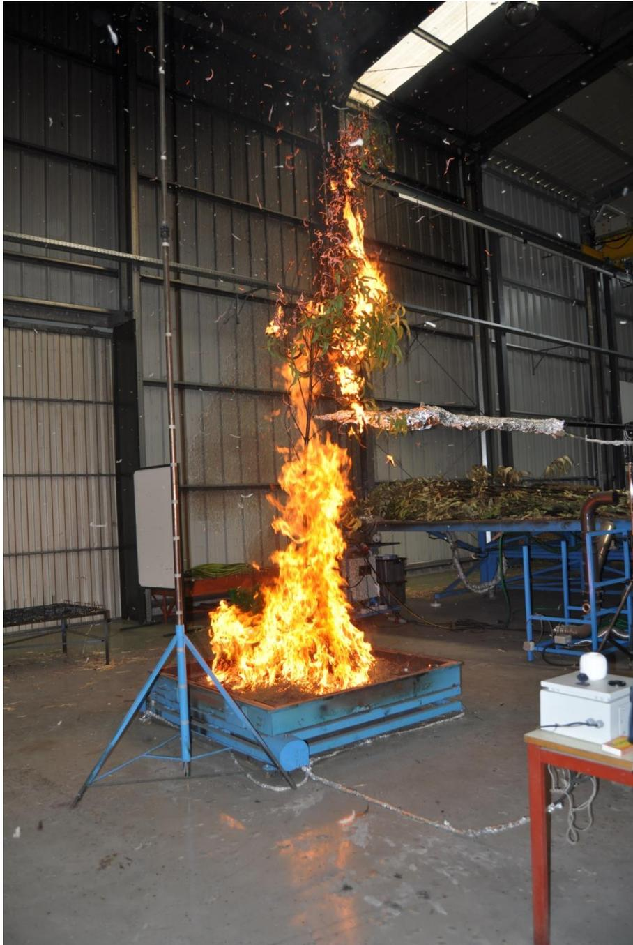
*Figure 5. An example of firebrand generated by the burning of trees*
