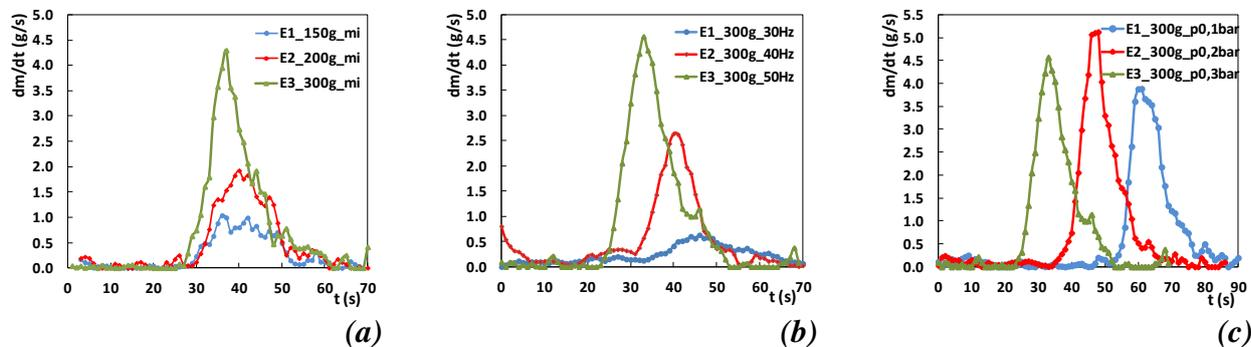
Figure 2. Plot of the rate of ember production  $dm/dt$  (g/s) as a function of time  $t$ (s). a) varying initial mass; b) varying flow velocity; c) varying gas pressure.
