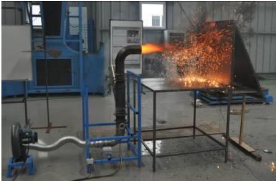
*Figure 1. Firebrand Generator Device*
