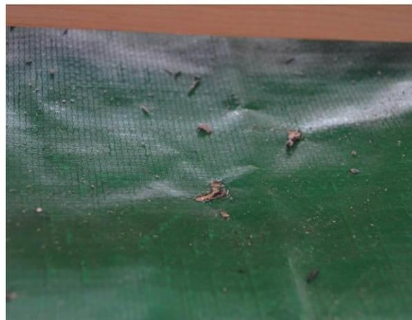
*Figure 6. Images of Sarking Placed Under Concrete Tiles (profiled tile) Taken Immediately after the Experiment was Completed. The Tiles have been removed [12].*
