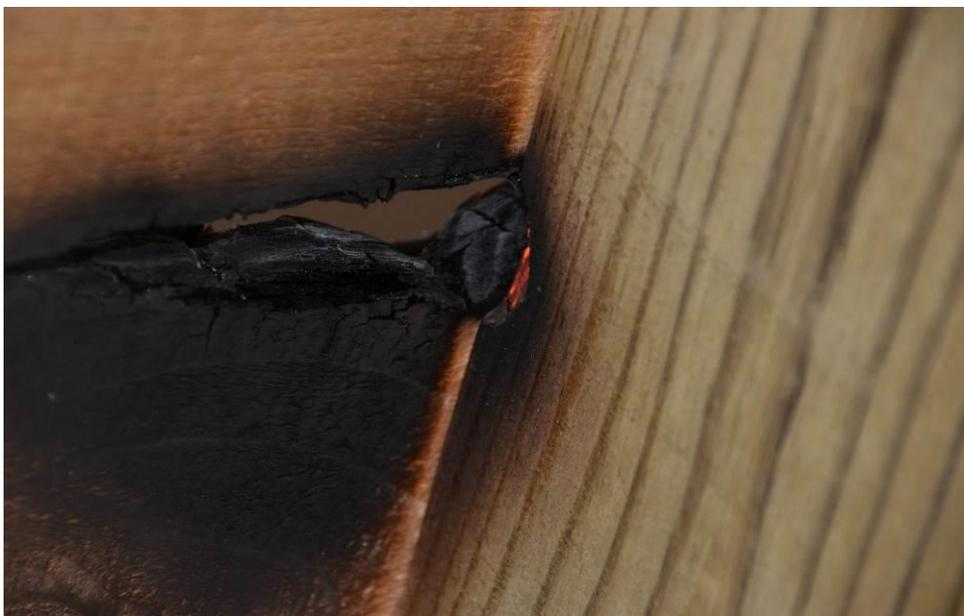
*Figure 3. Detail of the underside of the decking assembly (cedar). The ignition process was observed to spread to the wood supporting members [10].*
