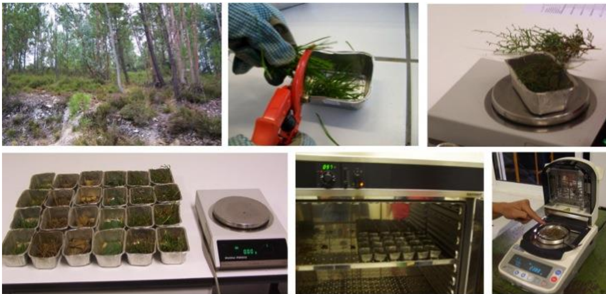
Figure 2. Sampling and determination procedures on the FMC research program of Lousã
