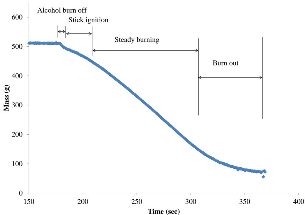
Figure 2. Sample raw data for 1.27-12-3-14 crib.
