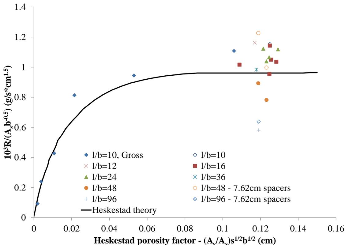
Figure 8. Burning rate including effect of crib-platform spacing.
