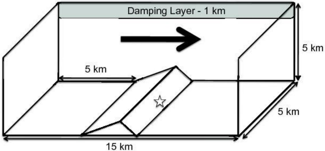
*Figure 1. Model domain showing the triangular mountain with its ridge line oriented perpendicular to the input wind field. The windward slope is inclined at  $20^\circ$  and the leeward slope is inclined at an angle of  $\alpha^\circ$  ( $\alpha = 35^\circ$  in the first set of simulations and is variable in the second set of simulations). The star on the leeward slope indicates the approximate location of the ignition used in the simulations.*
