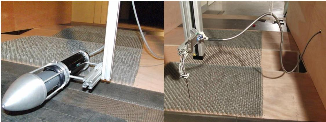
Figure 4. LDV on the left and FID on the right above the V-shaped forest model
