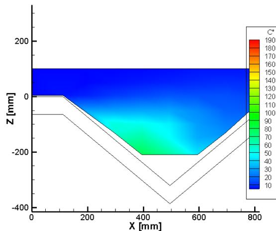
Figure 10. Concentration (ppm) of only wind side emitting for  $50^\circ$
