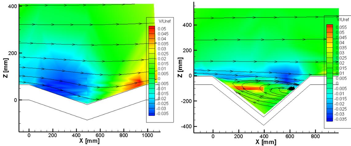
Figure 5. Vertical component of the velocity ( $V$ ) normalized by  $U_{ref}$  with streamlines of the velocity, for  $\alpha = 80^\circ$  on the left and  $\alpha = 50^\circ$  on the right
