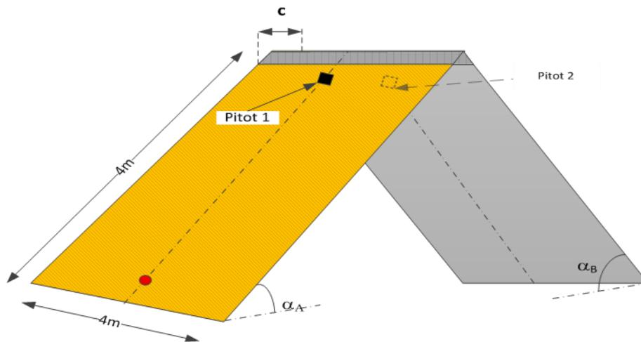
Figure 1. Schematic view of the ridge and the fuel break.
