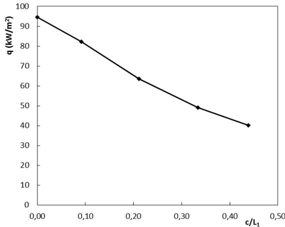
Figure 6. Computation of the net rate at which an infinitesimal element face B gains radiation due to the interaction of the flame in the side a for several values of  $c/L_1$ .
