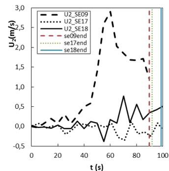
Figure 8. Flow velocity at positions P2 function of time for tests: SE 09, SE 17 and SE 18
