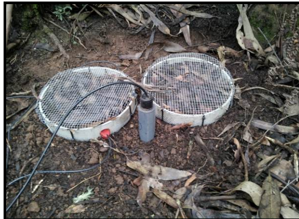
Figure 3. Two of the dead fine surface fuel sample packs used in this study to monitor fuel moisture. The left hand pack is fitted with three Vegetronix VH400 soil water content sensors, recording every 15 minutes. The right hand pack is used for manual gravimetric measurements during field site service visits. (Source: www.vegetronix.com ).
