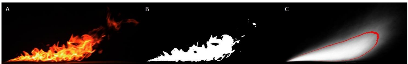
Figure 13. Image averaging technique used to determine flame geometry. (A) Still image from side-view camera (B) Black and white converted image using flame intensity threshold. (C) All black and white images averaged with pixel values between 0 and 1. A threshold line following pixels with value 0.48-0.52 are shown in red, identifying the average flame geometry.
