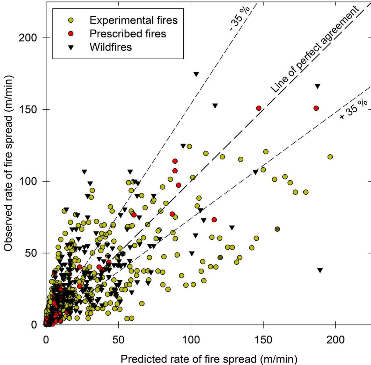
*Figure 2. Observed rates of fire spread versus model predictions by type of data involved in the 1278 pairs garnered from the 49 comparison studies as compiled by Cruz and Alexander (2013). The two dashed lines around the line of perfect agreement indicate the  $\pm 35$  percent error interval.*
