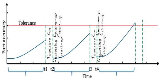
Fig. 1. Preventative calibration and adjustment at fixed rate
