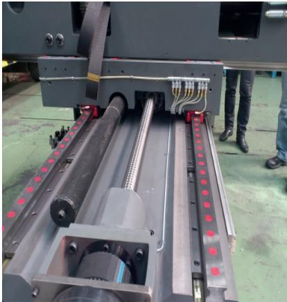
Figure V. Linear guides ball screw/nut
