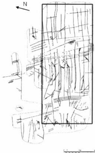
Fig. 5 – Map of a representative, strongly fractured granitic outcrop located in the area adjoining landfill facility. The rectangle bounds the selected domain for fractal geometry analysis.
